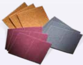
BearTex products consist of a non-woven web of nylon, impregnated with abrasive grain bonded with synthetic resins. This produces a cushioned, three-dimensional material which is extremely pliable and long lasting. The uniform dispersion of abrasive throughout the web provides a constant finish during use.
