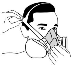
Place the respirator over the mouth and nose, then pull the head harness over the crown of the head.
