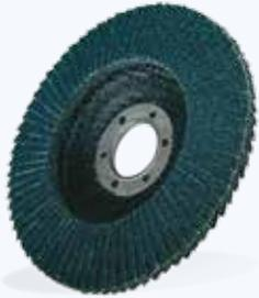
Norton Vulcan flap discs are manufactured with zirconium grain specially developed for use in flap discs providing greater aggression and fast stock removal, together with improved cotton cloth backing for better strength, flexibility and wear resistance.
