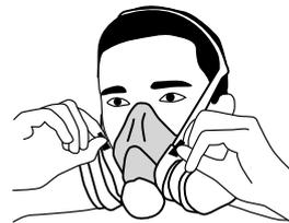
Tighten top strap by pulling on ends to obtain a secure and comfortable fit. Tighten bottom straps by pulling on ends or loosen by pushing out on buckle tab.
